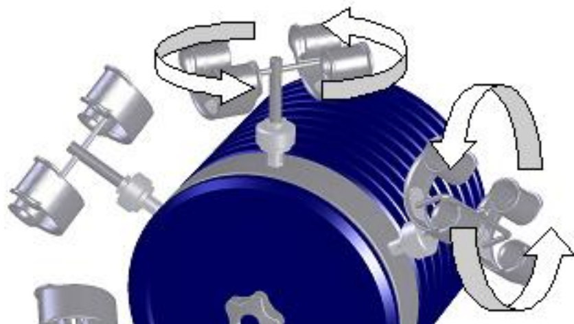
Fig. 3.6.2. Clip for watches that are wound up in one particular direction only
